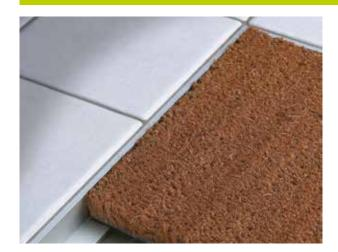
Reversible profile to create perimeters suitable for containing doormats. The profile accomodates the two most common doormat thicknesses of 11/16" and 29/32" - 18 and 23 mm. Installing the frame must be done at the appropriate height before the installation of the adjacent flooring material. The profile can also be installed using modular and sliding fixing brackets inside the slots.
